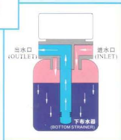
运行状态 Service State
