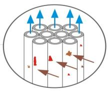
The feed water flows into hollow fiber membrane from external, water, small molecules, ions and etcpermeate to the internal membrane, so that come into permeability fluid, also solid particles are trapped in the outside of the hollow fiber membrane.
